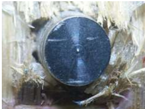
Figure 3: The bullet did not penetrate the laminated woven bamboo/woven E-glass
